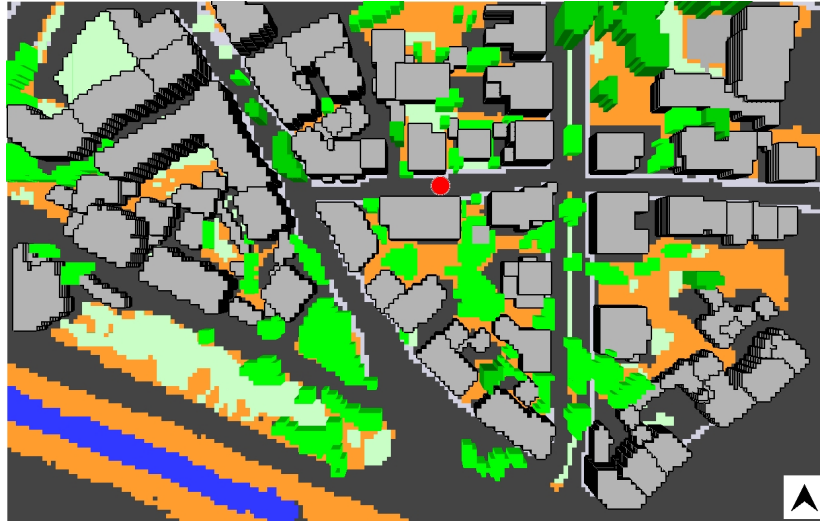
Figure 3: Model area Erbprinzenstrasse (372 x 236m). Buildings (grey), vegetation (green) and surface materials color coded. Red dot: measurement site.
