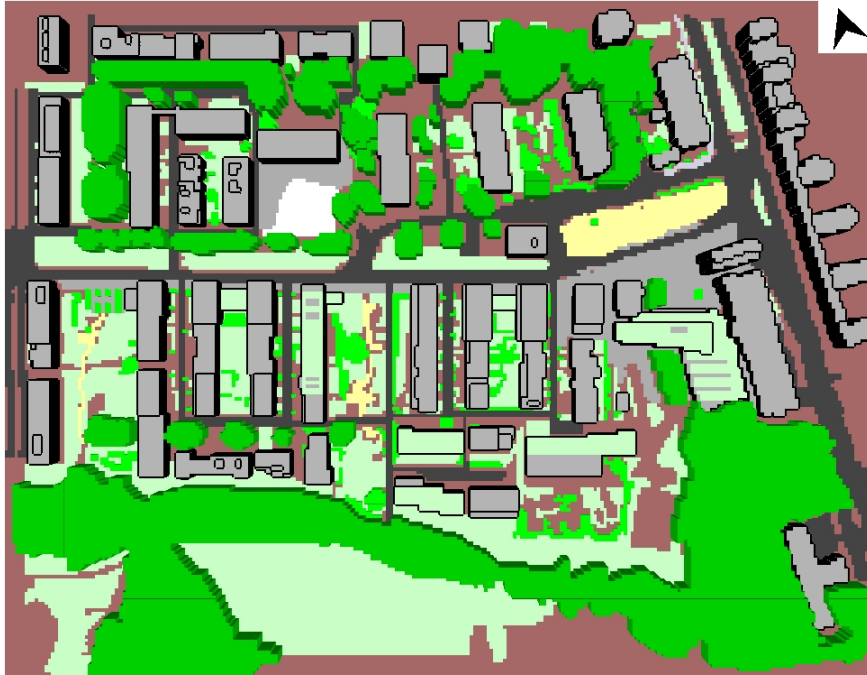
Figure 4: Model area Vauban (512 x 386m). Buildings (grey), vegetation (green) and surface materials color coded.
